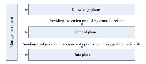
Figure 2: Independent system architecture of IOT
