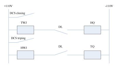
Figure 2 : HWJ and TWJ elementary wiring diagram
