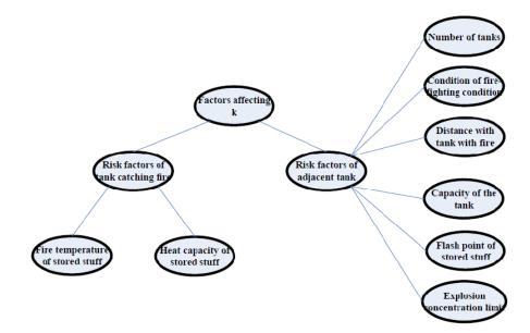
Figure 1: The determination of value k, by using layered structure instructions
