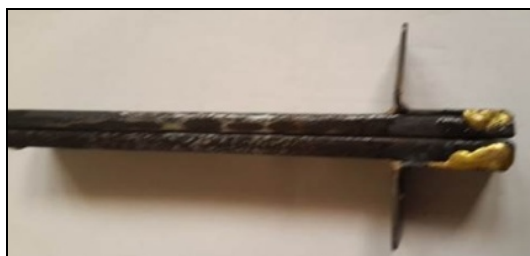
Fig. 4: Fabricated DCB specimen
