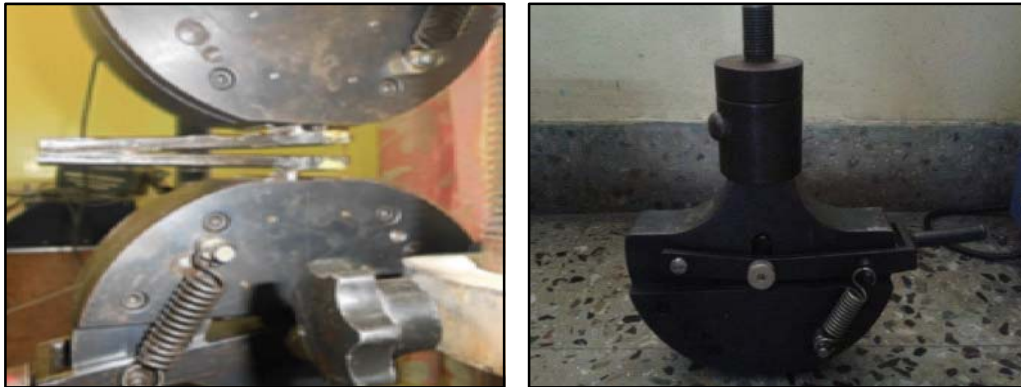
Fig. 5: Clamped DCB specimen and spring loaded fixture used in the test
