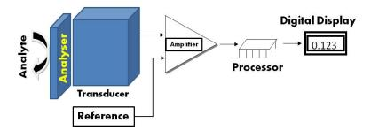
Fig. 1: Schematic diagram with basic components of biosensor
