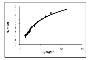
Fig. 1: Adsorption isotherm system: F-300-oxidised carbon-Ni<sup>2+</sup>
