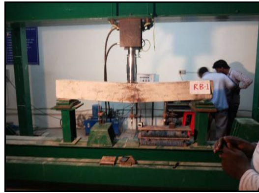
Fig. 5: Cracking pattern of RB specimen
