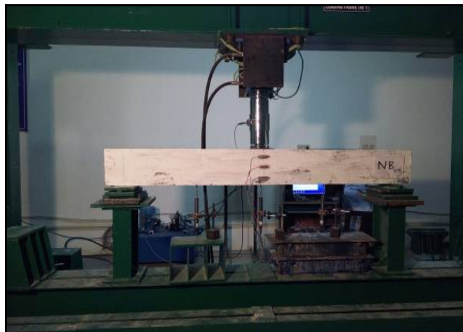
Fig. 2: Test setup of the control beam
