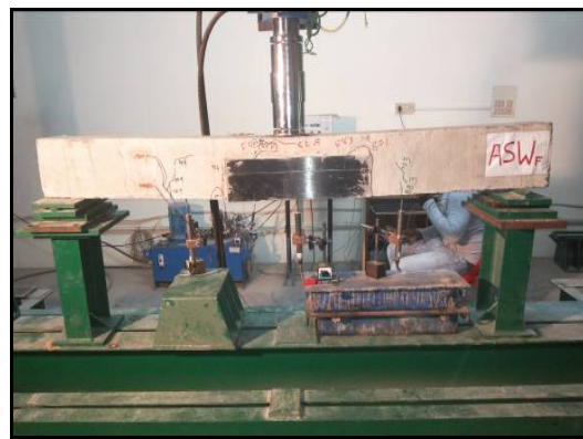
Fig. 7: Cracking pattern of ASW-F specimen
