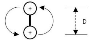
Figure 4 : Two similar charges being rotated with separation distance D creates quadrupole radiation.
