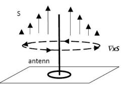
Figure 2 : Near field vectors around a dipole antenna on a metal sheet. Circle is insulating gap in sheet.
