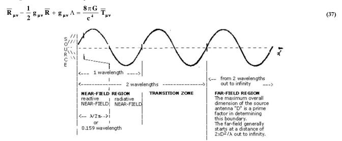
Figure 6: A diagram showing the relative scales of radiation zones around an antenna.
