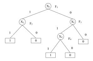
Figure 1 : The basic structure of BDD
