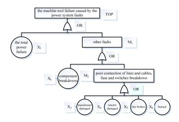
Figure 2 : The fault tree of the CNC machine tools caused by the power failure
