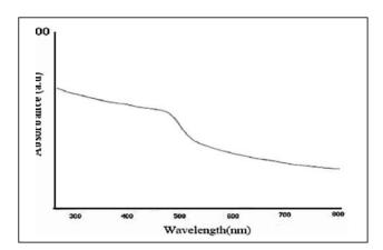
Fig. 1: UV-VIS absorption spectrum of CdS nanoparticles obtained by the offered route
