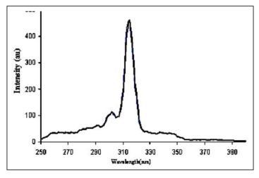
Fig. 4: PL emission spectrum of an absolute ethanol solution
