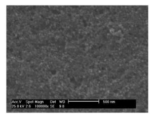
Fig. 3: SEM images of Cd prepared by the offered route.nanoparticles of the sample was recorded employing a double beam, Hitachi, Japan, applying quartz cuvettes of the optical path length 1 cm. The PL spectrum was achieved using Hitachi X530 fluorescence spectrophotometer with a 220 nm excitation line
