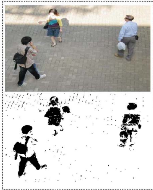
Figure 8: Moving object detection in outdoor scenes
