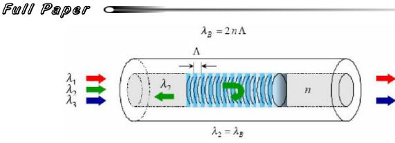
Figure 1 : Principle of operation of a fiber bragg grating
