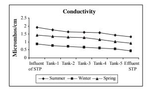
Fig. 3: Seasonal variation of electrical conductivity in sewage treatment plant
