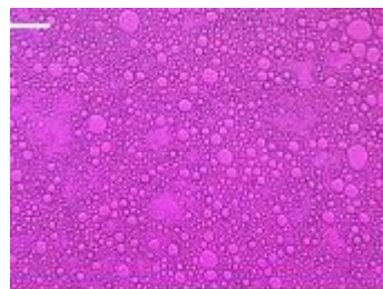
Figure 5: Light micrograph image of Brij 35 P based cream at 25 °C at 20 micron
