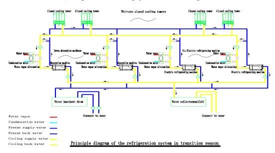
Figure 4 : Operation schematic diagram of cooling system in transition season
