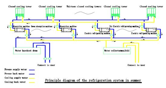
Figure 3 : Operation schematic diagram of cooling system in summer
