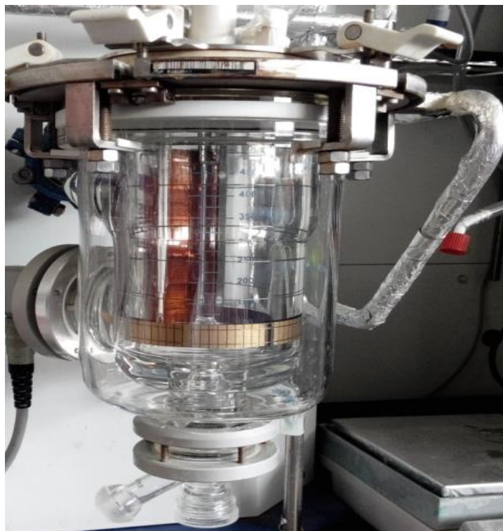
FIG. 2. RC1e-RTCal reactor with horizontal and vertical band of sensors.
