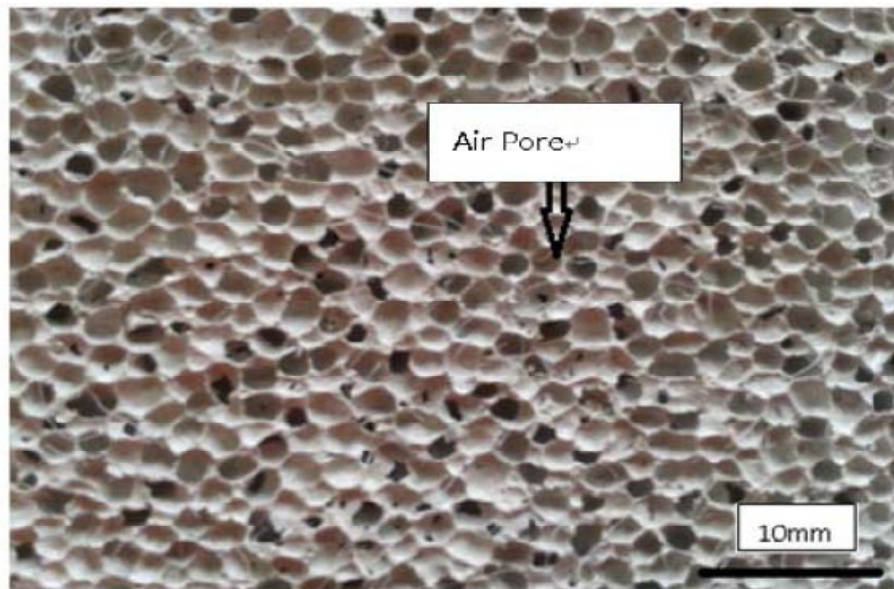
Figure 10: Section picture of foamed concrete through adding Ce^{4+}
