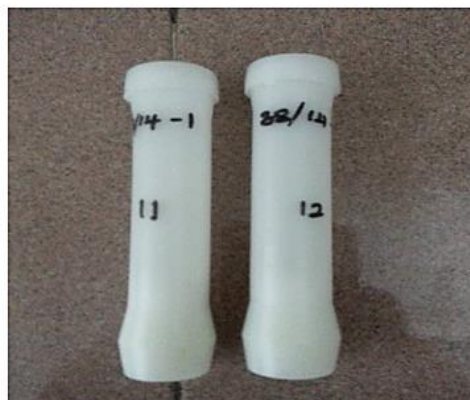
FIG. 2. (b) Pneumatic cylinders containing polyethylene vials.
