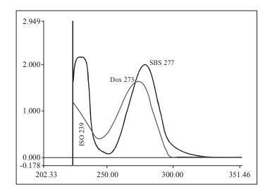
Fig. 2: UV Absorption spectrum of DOX and SBS laboratory mixture
