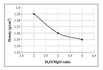
Fig. 1: Final product density as a function of the ratio H<sub>2</sub>O/MgO
