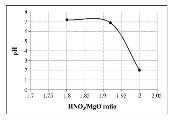
Fig. 2: Final product pH as a function of the ratio HNO<sub>3</sub>/MgO
