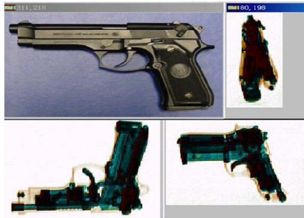
Figure 2: Image extraction by X-ray machine of the pistol from different angles
